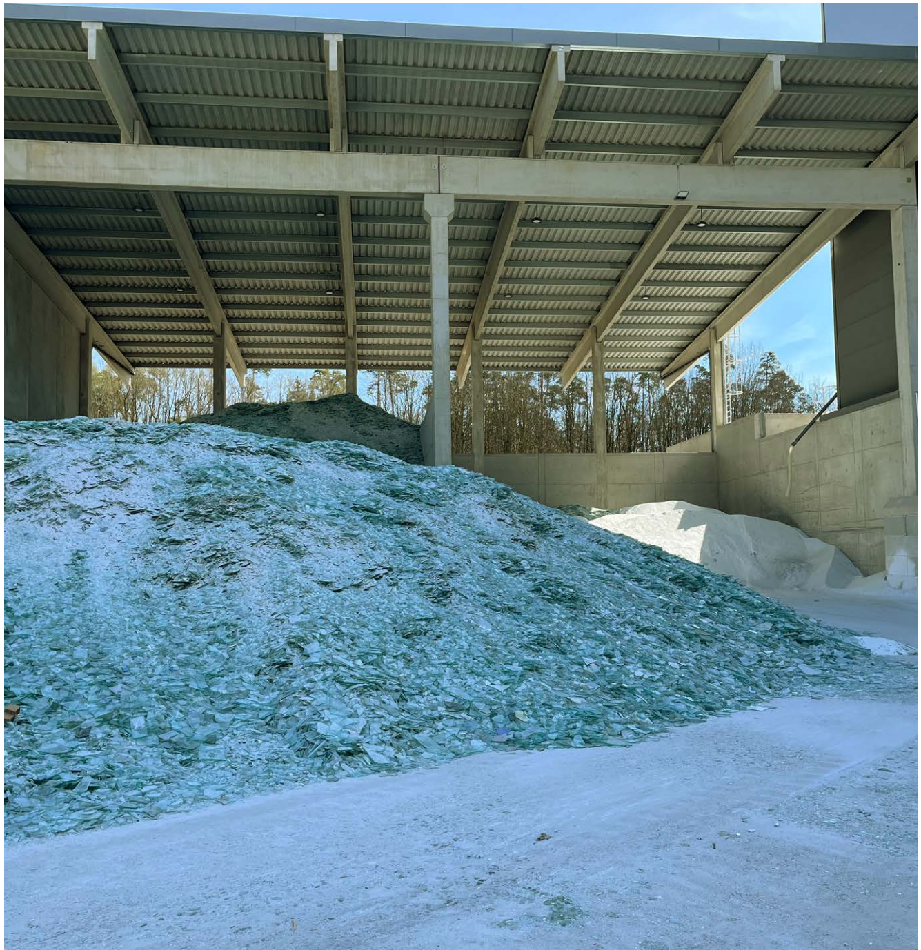
Upcycling: from flat glass cullet to reflective glass beads for improved road safety
